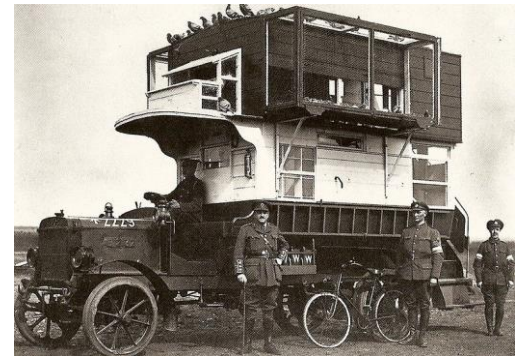
A B-type bus from London converted into a pigeon loft for use in Northern France and Belgium during the Great
